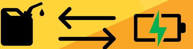
When batteries are low the X-HYBRID CUBE will automatically switch to its **diesel engine** and simultaneously recharge the battery whilst maintaining light output.
